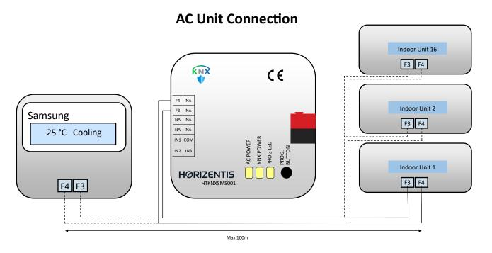
Supports connection of up to 16 indoor units; individual commands can be transmitted to connected units. When installing a gateway by using a cable longer than 10 m(32.80 ft), you must install the communication cable and the power cable separately. (Electrical interference can cause your gateway to malfunction.)
