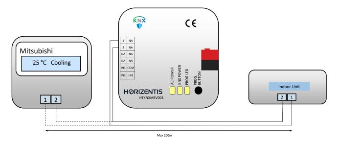
Wired remote controller must be in master mode if connected. In this case gateway must be set in slave mode from parameters.
