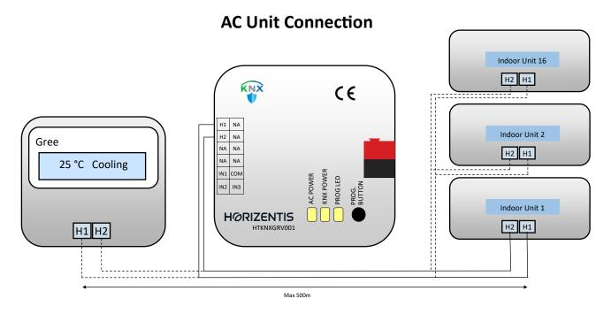
Wired remote controller must be in master mode if connected. In this case gateway must be set in slave mode from parameters. Supports connection of up to 16 indoor units; the same command is transmitted to all connected units.
