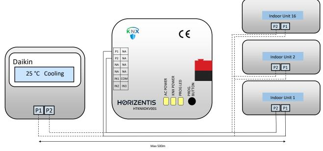
Wired remote controller must be in master mode if connected. In this case gateway must be set in slave mode from parameters. Supports connection of up to 16 indoor units; the same command is transmitted to all connected units.
